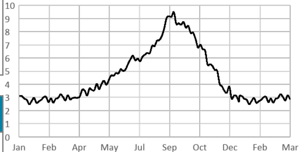
Corrosion rate of a Southeastern US surface water system: Corrosion rate in mils per year
