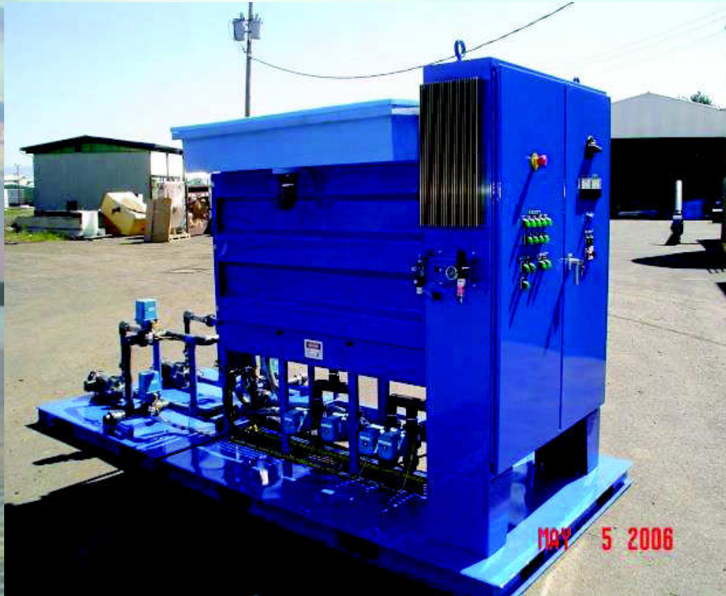
Powell Water 50 GPM Unit
