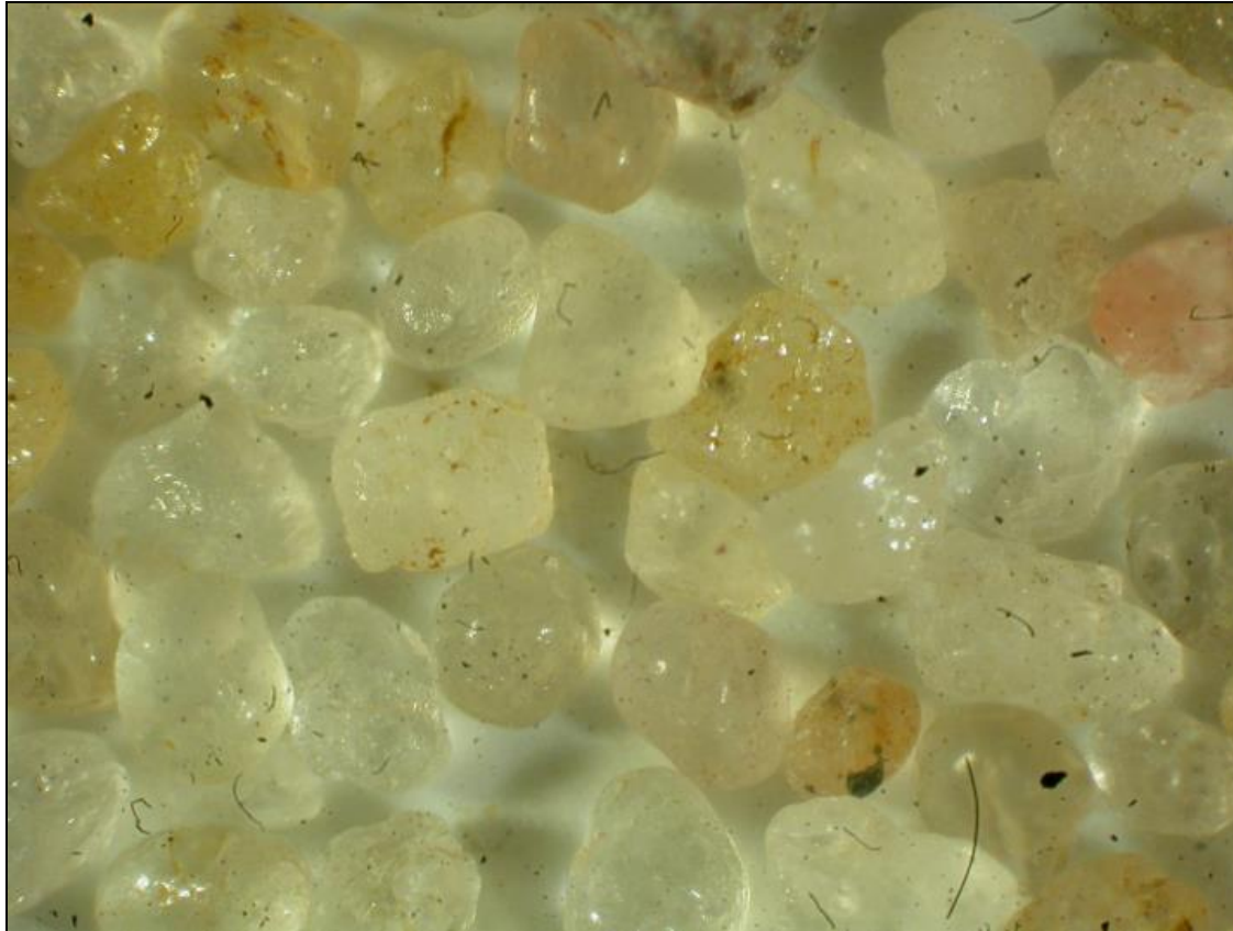
Filter sand with severely worn, rounded edges
