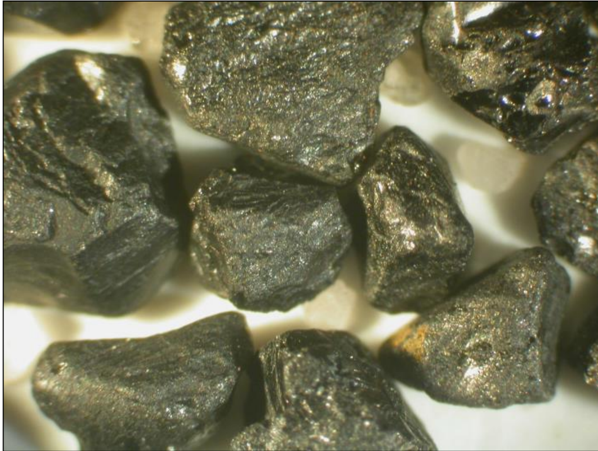
Washed anthracite media with worn, rounded edges
