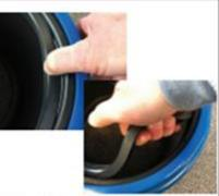
Use your thumb or other device to remove inner gasket layer.
