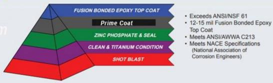
Multi-Clad Layered Coating System
