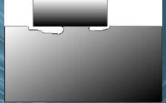
Poor Passivation at the Welds and Too Many Welded Components Leaving Weld Contaminants Behind can Lead to Erosion and Corrosion of the Weld
