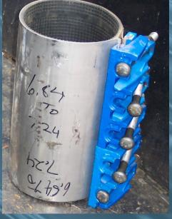
2 – 12 inches diameter (28 to 32 sizes to stock per width) .4" Range Means Many Sizes Mat gasket design Lifter bar Loose nuts/bolts or **Stud Welded bolts** All weld stainless or ductile lug design **Limited Range** Must conform to AWWA C 230-11
