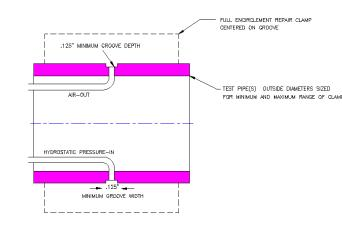
5.3.1.1 Test pressures. The minimum hydrostatic proof of design test pressure shall be 50 psi (345 kPa). For full-encirclement repair clamps where the purchaser has designated a rated pressure, the hydrostatic proof of design test pressure shall be 150 percent of the maximum rated pressure.
