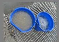
The material on the left shows sediment filled with material removed by the ice pig. The sample on the right shows material removed.
