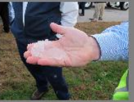
The ice slurry mixture acts as both a solid and a liquid. The consistency is very similar to a conventional slurry.
