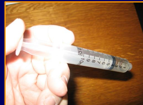
Syringe type pipettes suitable for use with jar test stock solutions
