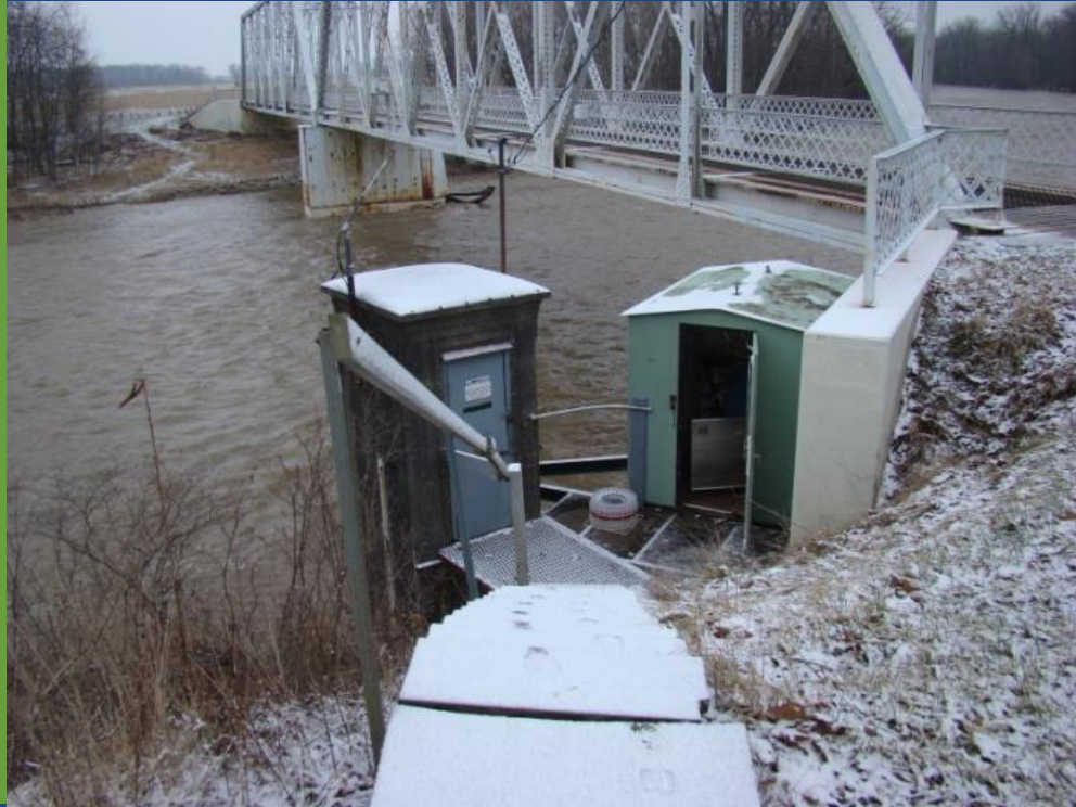
The stream gage and water quality sampling station at the Sandusky River near Fremont, Ohio (Site # 4198000)
