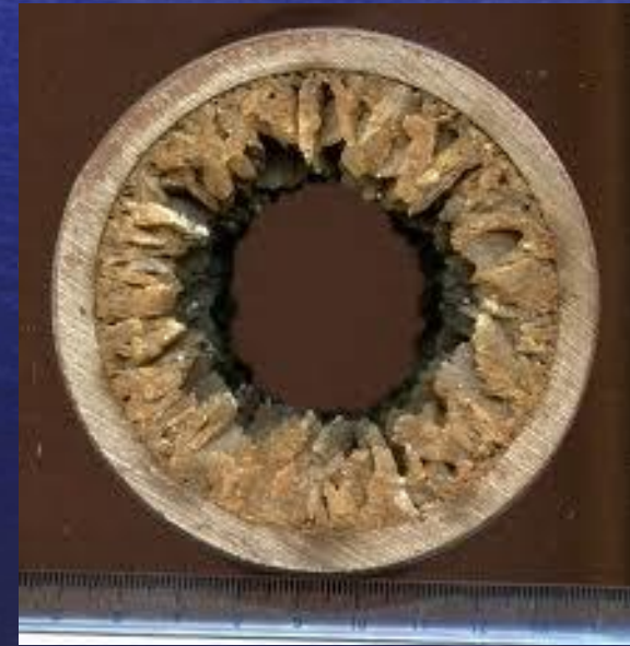
Pipe Scale still TENORM
