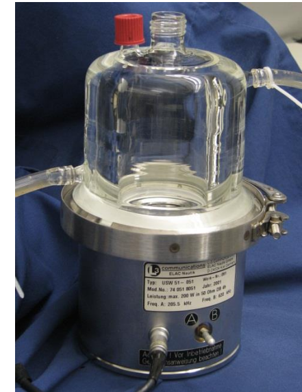
Frequency: 205 kHz Energy input: 45 W/L
