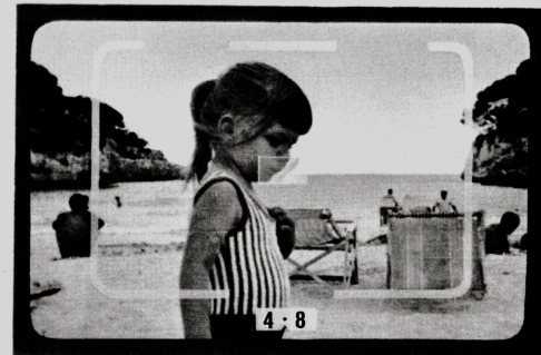
Your picture will show whatever is within the outline of the brightline finder at the time of exposure. In the picture above the selected aperture is 5.6 (dot between 4 and 8). The bright area in the center is the measuring patch of the rangefinder.
