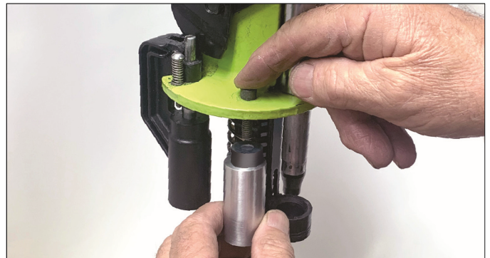
Fig. 5: With the spacer on top of the QuikLoader die, thread the knurled bolt into the QuikLoader die. Hand tighten only.
