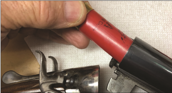
Fig. 1: Because standard shotshells are the same diameter as the chamber's mouth, they require precise entry to feed well and easily.
