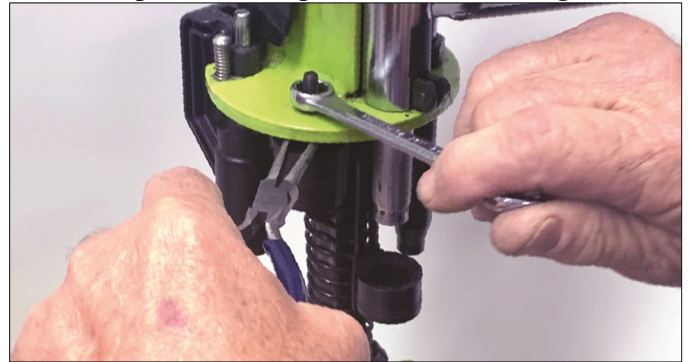
Fig. 4: A thin 7/16" open end wrench or needle nose pliers is used to secure the nut below the tool plate as another 7/16" wrench is used to loosen the nut on top of the tool plate.
