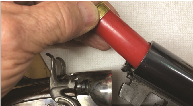
Fig. 2: Shells that have been shaped by a QuikLoader die can enter the chamber more easily and at a steeper angle. QuikLoader improves feeding in Winchester Model 97 pump shotguns, too!
