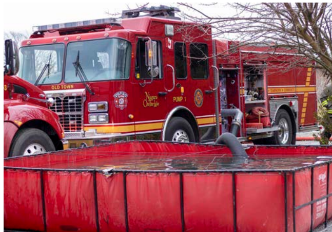
NOTL Fire and Emergency Services use portable ponds as a water source, instead of fire hydrants, when fighting back flames in rural parts of town. FILE
