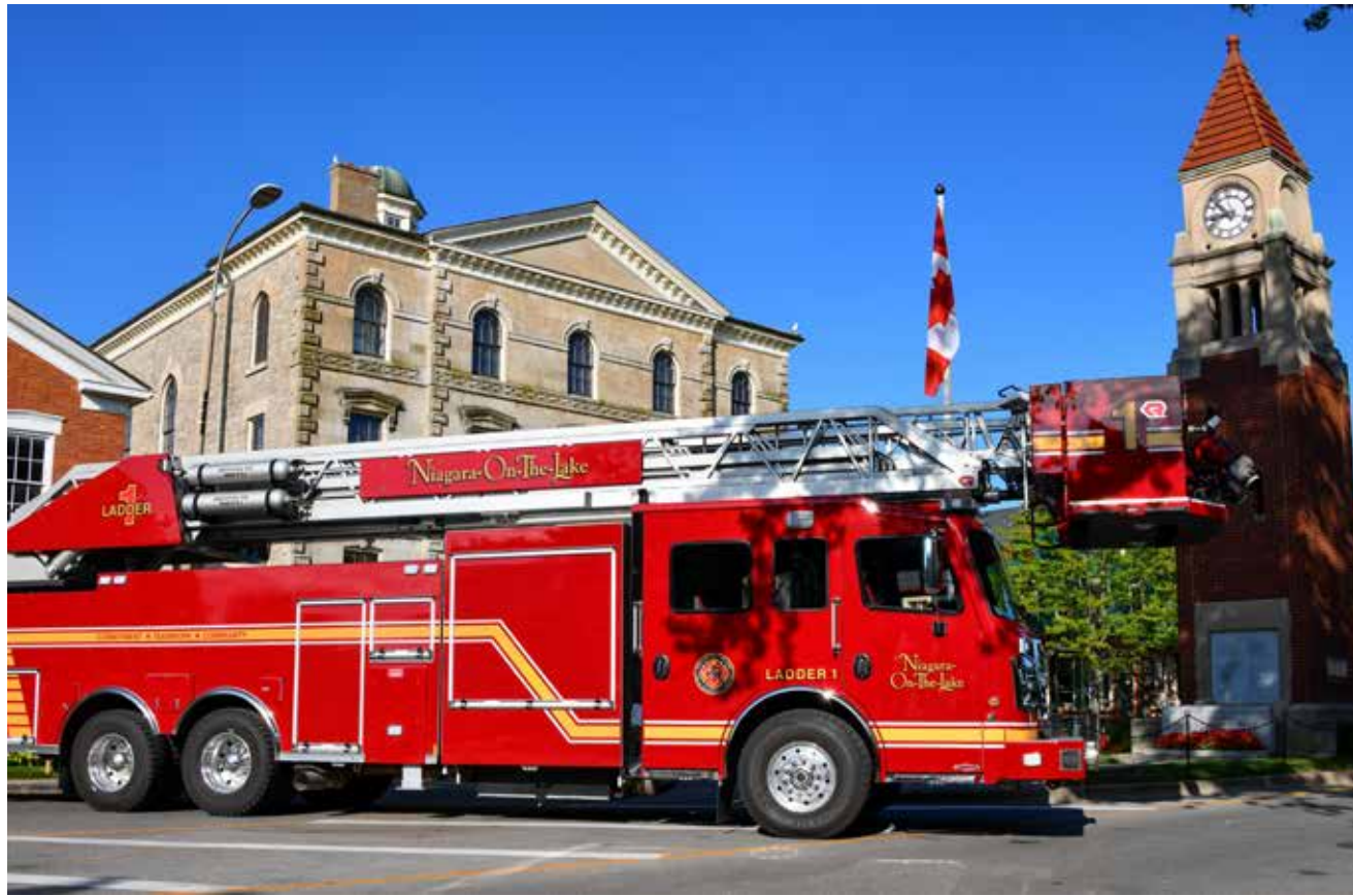
The Niagara-on-the-Lake fire department's new 2019 Rosenbauer Cobra 101' aerial platform fire truck. KYLE TAYLOR
