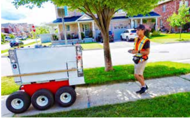
An operator from Top Hat Robotics conducts a sidewalk inspection on Wright Crescent in the Niagara on the Green neighbourhood in Glendale on Monday afternoon. Two robots were patrolling the area looking for sidewalk defects. If the robot detects one, the sidewalk is then marked with spray paint for future maintenance by town staff. Using robotic technology will speed up inspections and allow staff to do other tasks, the town says. STEVE HARDAKER PHOTO
