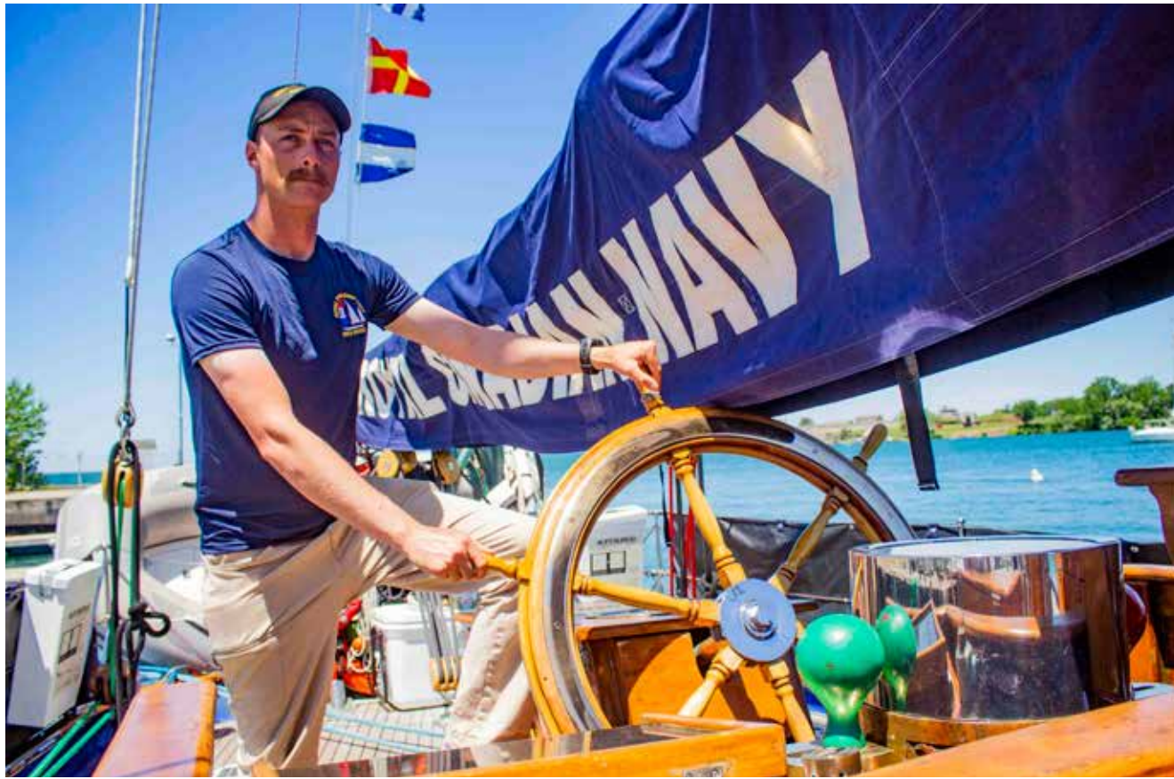
Executive officer of the HMCS Oriole James Craigie demonstrates how the helm is positioned in large ships. The helmsman typically has one foot on either of the side blocks and holds the helm of to the side of his body. EVAN SAUNDERS
