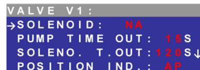
To configure the type of SOLENOID valves that the VOLTA Controller is connected to, select the option by navigating using the arrow buttons and press the ENTER button and you will see the current value flashing; in this case NA, modify the value using the arrow buttons. Once the desired value is reached, press the
