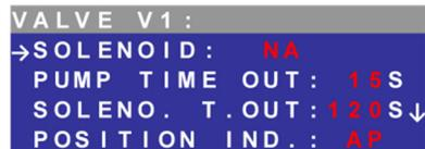
In this screen you can configure the type of SOLENOID, pulse duration of the hydraulic pump called PUMP TIME OUT, pulse duration to the solenoid called SOLENOID TIME OUT and configure whether a position indicator is connected or not.
