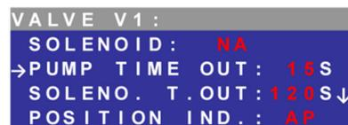
To set the maximum duration of the energy pulse that the VOLTA Controller will deliver to the hydraulic pump named PUMP TIME OUT, select the option by navigating using the arrow buttons and press the ENTER button and you will see the current value flashing, in this case 15 seconds; change the value using the
