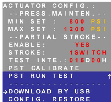
In this screen you can download to a pen drive the data stored in the VOLTA Controller's memory regarding time and speed measurements and results arisen from the PST or TST run by the VOLTA Controller.
