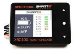
to like a little higher voltage for a storage charge. This could be from the controller that is built right into the battery itself or just the chemistry. Either way this is a good time of year to take your battery checker and go to each flight pack you have and give them a quick check. There is always a slight internal discharge taking place. Now this internal discharge does get worse depending on how you treat
