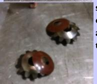
of back lash is required. If you feel the gears are too snug and need a bit more clearance; disassemble the case and stone or grind the side gear shims and start all over until you are satisfied. Now that the gear case is assembled set it aside and cover it with a clean shop towel.
