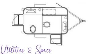
Fresh Water Tank: 86 gallon | Black Water Tank: 225 gallon Length: 14.5' (with tongue) | Width: 8' (with stairs) | Height: 12' Water Requirement: Garden hose spigot Power: (1) 110v20amp circuits
