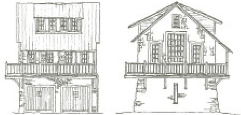
Carriage House Side & Front Elevation
