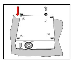
**1.** Place the projector upside down on a soft cloth and remove or lower the feet as much as possible.
