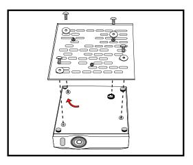
2. Align and attach Universal Tray to the projector mounting inserts with the supplied Machine Screws and Washers.
