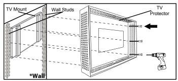
Guide TV Protector through TV mount using it as reference for positioning.
