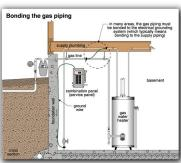
Only one grounding rod (grounding electrode) was observed on the property. Current building standards require installation of two grounding electrodes. The presence of a proper grounding electrode system should be verified or a proper grounding electrode system should be installed for safety. **This house predates the adoption of this standard; however, this should be corrected for safety reasons.**
