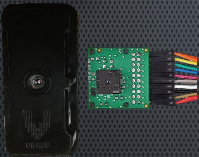
Fig.2 Form factor of camera unit & thermal core
