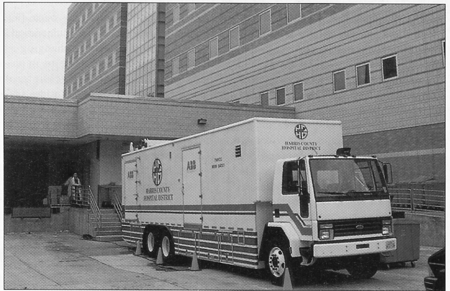
In Harris County, Texas, Bentau and LBJ hospitals are sharing a Sanitec Inc. mobile microwave disinfection system to dispose of a combined 8,000 to 9,000 pounds per day of medical waste. All surgical waste except organs and body parts (which are packaged and sent to an incinerator) are dumped by an automatic hoist into the in-feed hopper at the top of the trailer. The on-board processing system includes a shredder that can reduce sharps and syringes, gowns, towels, plastic and other waste into a uniform size for disinfection in a steam treatment chamber. Next material is carried by a screw conveyor to a series of microwave generators, and discharged only after a chart recorder substantiates that disinfection is complete. (photos courtesy Sanitec, Inc., West Caldwell, NJ)
