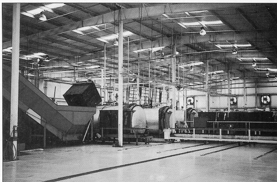
Medical waste received at Applied Recovery is treated using three autoclaves that operate at 275 to 280 degrees under 48 psi of steam pressure. All waste is shredded prior to being loaded onto trailers for transport to an approved landfill.
