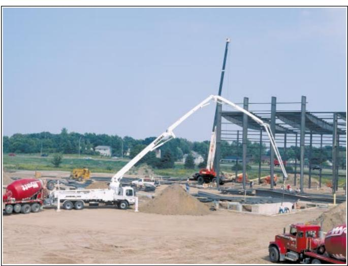
Only Schwing makes the longest boom reach available on a three-axle truck with the 39-meter model. Efficient and maneuverable, the 39-meter boom length is ideal for concrete pumpers, ready-mix producers and concrete contractors. This well-balanced unit employs X-Style outriggers for easy, compact set-up in crowded condi-
