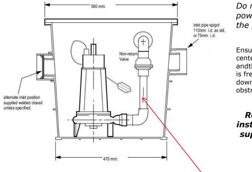
*Do not use the power cable to lift the pump.*
