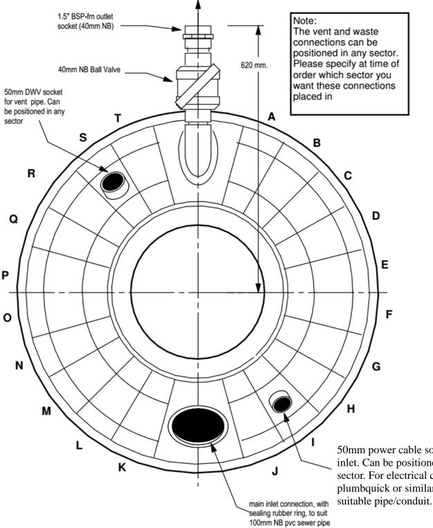
50mm power cable socket pipe inlet. Can be positioned in any sector. For electrical cable, use plumbquick or similar to connect to
