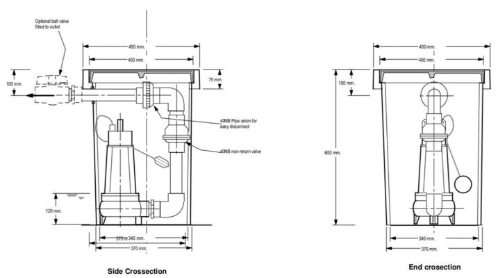
65 Litre Storm Water Pump Station- For Pump Models TP0118- VH100/40MF
