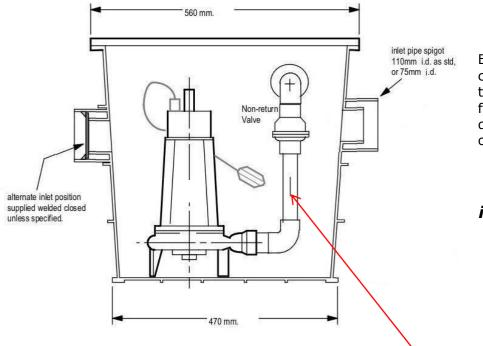
Ensure that the pump is centred in the tank, and that the float switch is free to move up and down without obstruction.
