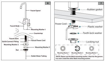
Connect one end of the Blue purified water PE-tube (BLUE) to the faucet by pushing it into the quick-connect fitting. Secure the PE-tube with the safety clips (see chapter How to use the quick-connect fittings).
