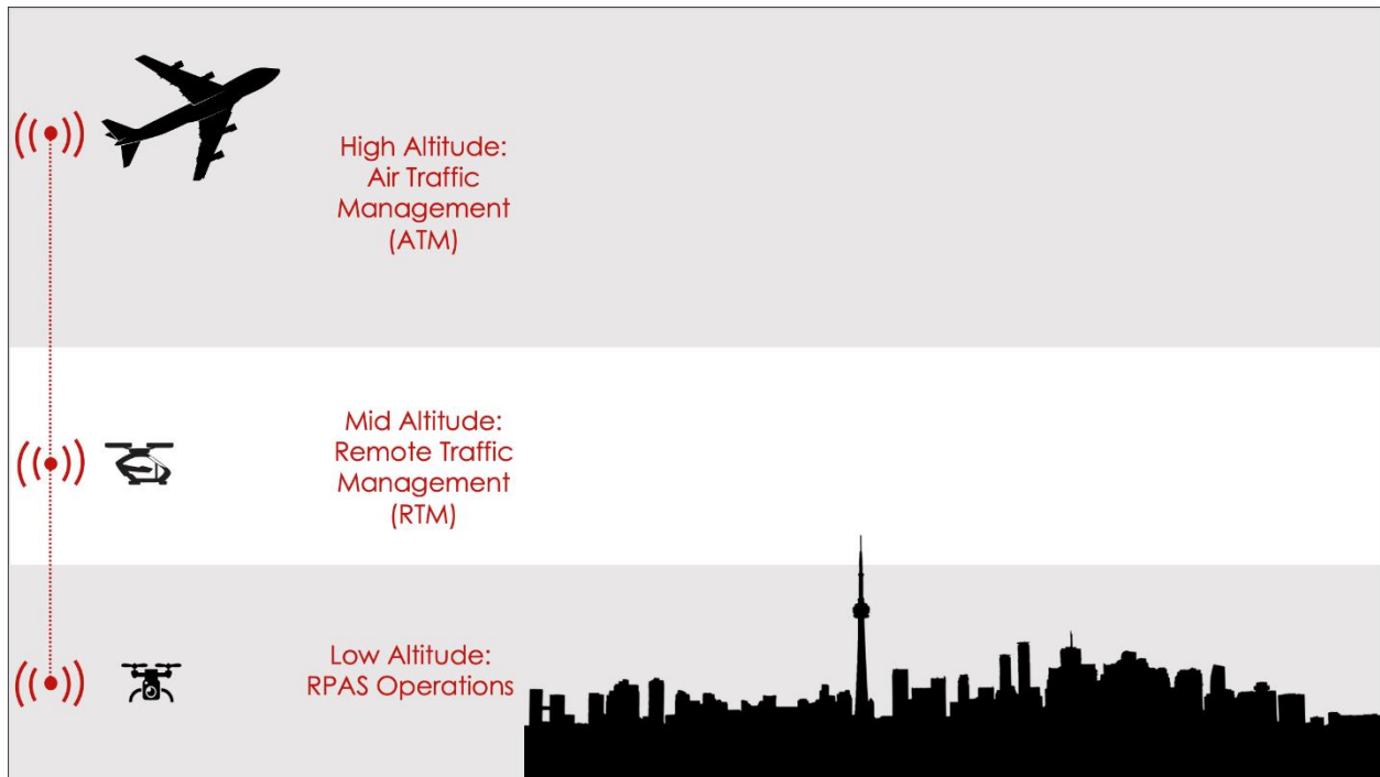
Figure 15 - Airspace layers help to organize traffic into manageable segments for Advanced Air Mobility to work harmoniously in today's aviation environment.
