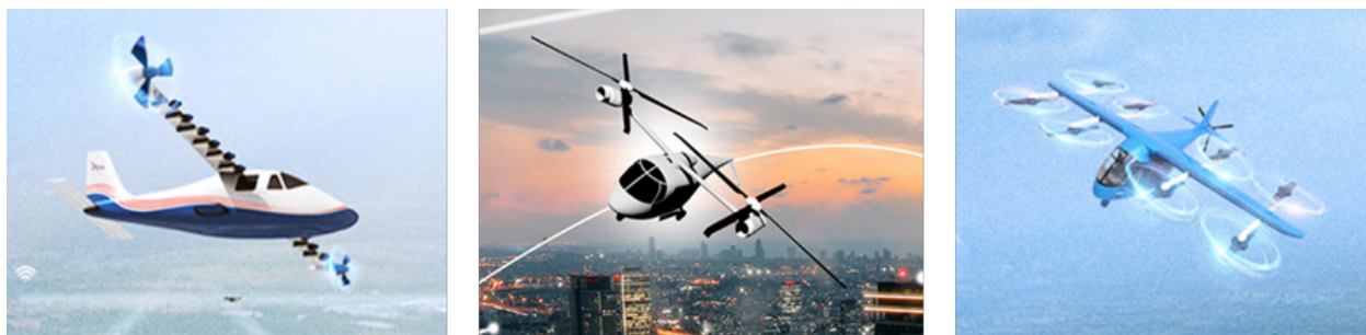
Figure 7: Example Vectored Thrust 39 , Lift and Cruise 40 , and Multicopter 39 Aircraft
