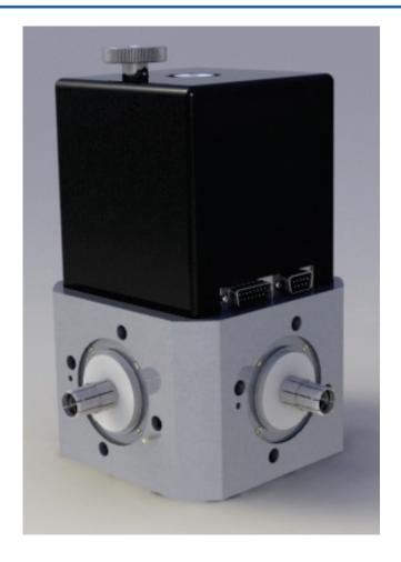
The models SW 158.01, SW 158.02 and SW 158.03 are motor-driven, two-way coaxial transfer switches designed to change coaxial connections with a minimum off-air-time. Mainly they are used for switching transmitters, antennas, dummy loads and other peripheral equipment in situations when broadcasting procedures are modified, when there is need for emergency repair, or during scheduled maintenance.
