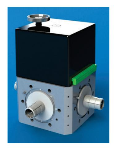
The models SW 318.01, SW 318.02 and SW 318.03 are motor-driven two-way coaxial transfer switches designed to change coaxial connections with a minimum off-air-time. Mainly they are used for switching transmitters, antennas, dummy loads and other peripheral equipment in situations when broadcasting procedures are modified, when there is need for emergency repair, or during scheduled maintenance.
