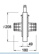
Gas barrier with silicone O-ring and stainless steel hardware set.
