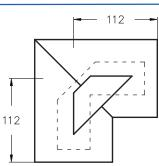
Miter elbow 90°-unflanged, reinforced outside, copper construction. Includes only one unsupported inner conductor.
