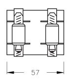
Line coupling for connection of unflanged lines. No inner conductor connector. Includes two stainless steel hose clamps (does not increase outer conductor length).
