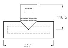
Tee assembly, unflanged, copper construction. Includes only supported inner conductor.
