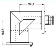
Miter elbow 90°, swivel EIA flanges on both ends, reinforced outside, brass and copper construction. Includes <u>supported</u> inner conductor, anchor insulator conductor connector, silicone O-ring and stainless steel hardware set.
