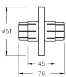
Anchor insulator conductor connector, for EIA flange connection, silver plated. *Short version*.
