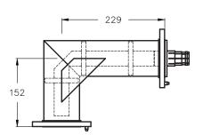
Miter elbow 90-unequal legs, swivel EIA flanges on both ends, reinforced outside, brass and copper construction. Includes supported inner conductor, one anchor insulator conductor connector, silicone O-ring and stainless steel hardware set.
