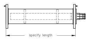
Line assembly, flanged with fixed and swivel flange. Brass and copper construction. Includes one anchor insulator conductor connector, silicone O-ring and stainless steel hardware set.
