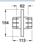
Anchor insulator conductor connector, for EIA flange connection, silver plated. *Short version*.
