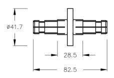
Anchor insulator conductor connector, for EIA flange connection, silver plated. *Standard lenght*.
