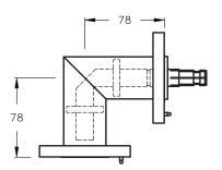
Miter elbow 90°, swivel EIA flanges on both ends, brass and copper construction. Includes <u>supported</u> inner conductor, anchor insulator conductor connector, silicone O-ring and stainless steel hardware set.
