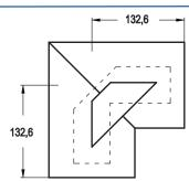
Miter elbow 90-unflanged, reinforced outside, copper construction. Includes only one <u>unsupported</u> inner conductor.
