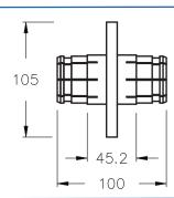
Anchor insulator conductor connector, for EIA flange connection, silver plated. *Standard lenght*.
