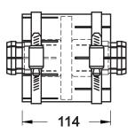
Line coupling for connection of unflanged lines. Includes supported inner conductor connector and two stainless steel hose clamps.
