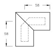
Miter elbow 90°-unflanged, copper construction. Includes only one unsupported inner conductor.
