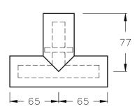
Tee assembly, unflanged, copper construction. Includes only supported inner conductor.
