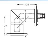
Miter elbow 90°, swivel EIA flanges on both ends, reinforced outside, brass and copper construction. Includes <u>supported</u> inner conductor, anchor insulator conductor connector, silicone O-ring and stainless steel hardware set.
