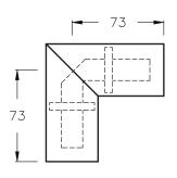
Miter elbow 90-unflanged, long legs, copper construction. Includes only one supported inner conductor.
