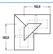
Miter elbow 90-unflanged, long legs, reinforced outside, copper construction. Includes only one supported inner conductor.
