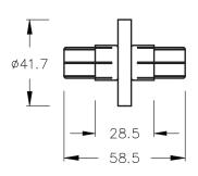
Anchor insulator conductor connector, for EIA flange connection, silver plated. *Short version*.
