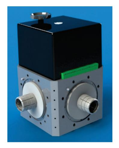
The models SW 412.01, SW 412.02 and SW 412.03 are motor-driven two-way coaxial transfer switches designed to change coaxial connections with a minimum off-air-time. Mainly they are used for switching transmitters, antennas, dummy loads and other peripheral equipment in situations when broadcasting procedures are modified, when there is need for emergency repair, or during scheduled maintenance.
