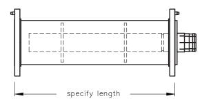
Line assembly, flanged with fixed and swivel flange. Brass and copper construction. Includes one anchor insulator conductor connector, silicone O-ring and stainless steel hardware set.
