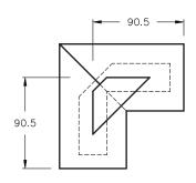
Miter elbow 90 unflanged, reinforced outside, copper construction. Includes only one unsupported inner conductor.
