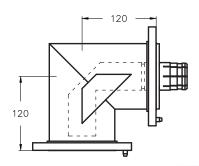
Miter elbow 90°, swivel EIA flanges on both ends, reinforced outside, brass and copper construction. Includes <u>unsupported</u> inner conductor, one anchor insulator conductor connector, silicone O-ring and stainless steel hardware set.
