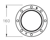
Fixed EIA flange with silver solder ring insert for silver brazing to outer conducting tubing.
