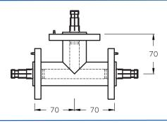
Tee assembly, swivel EIA flanges. Includes three anchor insulator connectors, O-rings and hardware sets.
