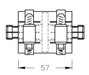
Line coupling for connection of unflanged lines. Includes supported inner conductor connector and two stainless steel hose clamps.
