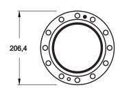
Fixed EIA flange with silver solder ring insert for silver brazing to outer conducting tubing.
