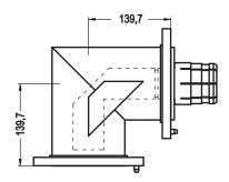
Miter elbow 90°, swivel EIA flanges on both ends, reinforced outside, brass and copper construction. Includes <u>unsupported</u> inner conductor, one anchor insulator conductor connector, silicone O-ring and stainless steel hardware set.
