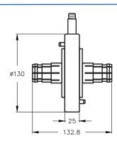
Gas barrier with silicone O-ring and stainless steel hardware set.
