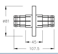
Anchor insulator conductor connector, for EIA flange connection, silver plated. *Standard lenght*.
