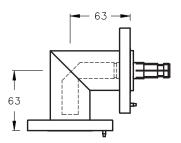
Miter elbow 90°, swivel EIA flanges on both ends, brass and copper construction. Includes <u>unsupported</u> inner conductor, one anchor insulator conductor connector, silicone O-ring and stainless steel hardware set.
