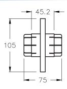
Anchor insulator conductor connector, for EIA flange connection, silver plated. *Short version*.
