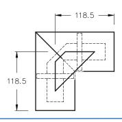
Miter elbow 90 unflanged, long legs, reinforced outside, copper constuction. Includes only one supported inner conductor.
