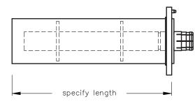
Line assembly, one end fixed flanged. Includes one anchor insulator conductor connector, silicone O-ring and stainless steel hardware set.
