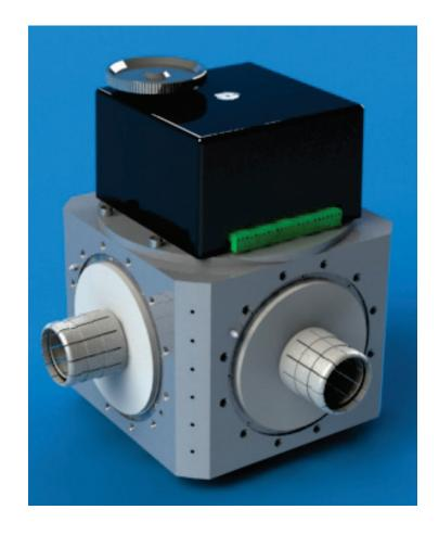
The models SW 618.01, SW 618.02 and SW 618.03 are motor-driven two-way coaxial transfer switches designed to change coaxial connections with a minimum off-air-time. Mainly they are used for switching transmitters, antennas, dummy loads and other peripheral equipment in situations when broadcasting procedures are modified, when there is need for emergency repair, or during scheduled maintenance.
