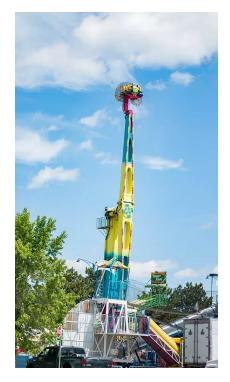
The G - Force can accommodate up to 8 passengers (4 each vehicle) and they are seated on free spinning vehicles back to back, with dangling legs. Each vehicle is equipped with a shoulder bar closed by a double locking device. Vehicles can perform a 360 degree rotation and their variable speed can reach a max speed of 62 mph.
