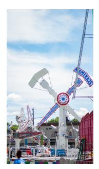
The ride is made up of a central column supporting two swinging arms. On each side of the arms a vehicle is fixed,
