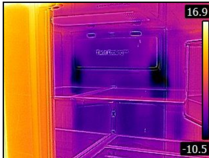
Refrigerators thermal scanned to confirm walls are cold at time of inspection.
