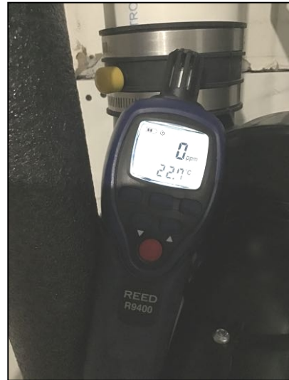
Carbon monoxide reading was ZERO during testing of tank.
