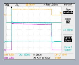
**100 kV, 42 A, 2 ms Output Pulse** from the modulator pictured above into a resistive load. Scope shows command (yellow, 5V/div), current (blue, 10 A/div); and voltage (purple, 22 kV/div).
