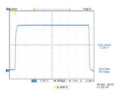
**108 kV, 3.5 ms, 0.07% Flattop Pulse** of DTI's Hybrid System into a Thales TH2179A klystron during site acceptance testing at IN2P3, 18 December 2015.
