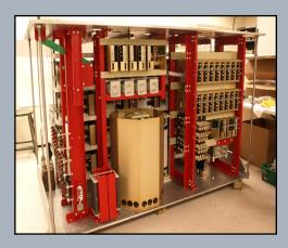
**DTI Marx Modulator.** Twenty 6 kV "core" switch modules erect a 120 kV output pulse when placed in series. Sixteen 900 V "corrector" switch modules address droop over the 1.5 ms pulsewidth.
