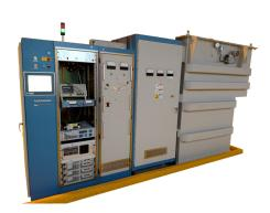
**DTI Hybrid System.** This ESS-class klystron test stand leverages a solid-state driven pulse transformer to provide a stable high voltage pulse (115 kV) over 3.5 ms.
