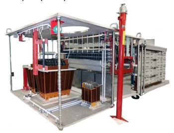
Fig. 4. 250 MW Modulator construction, with the pulse transformer in front, and the switch modules at the rear. The energy storage capacitors are visible in the center section. This entire assembly is submerged in an oil tank for operation.
