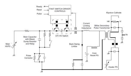
Fig. 2. Simplified modulator schematic. Directly switching 35 kV on the primary simplifies the pulse transformer and improves the risetime compared to higher step-up ratio designs. Series IGBT switches have inherent redundancy such that several modules may fail before system performance is affected.
