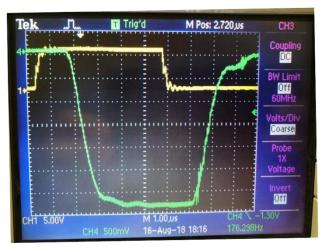
Fig. 3. Site Test of System #1 at Daresbury Laboratory. Pulse conditions were 385 kV, 440 A, 4 microseconds flattop, and without the pulse flattening circuit in operation. Scale is 1 microsecond per division. Trace 1 – Pulse Command; Trace 4 – Voltage.
