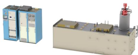
Fig. 1. 250 MW Peak Power CLARA Klystron Modulator System. High voltage solid-state switching allows a simple and reliable modulator with extremely high pulse fidelity and stability. One rack houses low voltage circuitry and controls (left) while a double-wide rack houses DTI's standard high voltage power supply and step-up AC transformer (center), allowing standard US 480 VAC input to the HVPS from 380 VAC British power.
