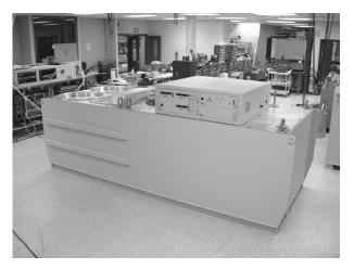
FIGURE 3. 500 kV, 500 A hybrid modulator
