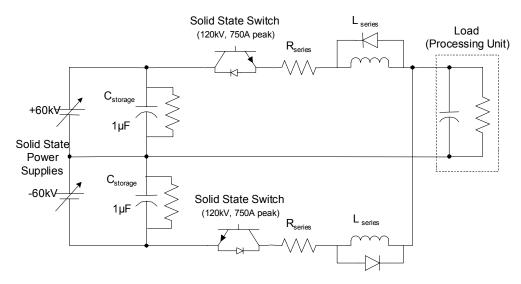
FIGURE 2. Bipolar PEF system block diagram
