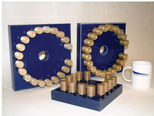
Figure 5. Three DTI 10 kV solid-state switchplates.
