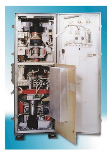
Figure 3. AN/SPG-60 radar cabinet. DTI's upgrade kit is installed in the lower compartment.
