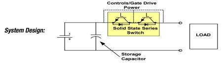
• A "hybrid" modulator solution. Combining DTI's advanced solid-state switches with a state-of-the-art pulse transformer in a very compact footprint, these designs are most cost-effective for low duty cycle systems. They deliver complex pulse trains, such as pulsed pairs and bursts, with extremely good pulse shape and stability for all pulses in a group.
