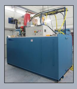
**DTI Commercial Klystron Transmitter System.** This system delivers up to 14 MW peak power with an average power of 500 kW.
