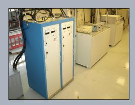
**DTI Klystron Transmitter.** This modular rack model gives greater system availability and klystron reliability than traditional designs, reduces the available arc energy, and simplifies mod-anode voltage control. This system operates at peak 100 kV and 50 A, with a pulse-width of 2 ms.
