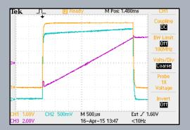
**Output pulse** from a Klystron modulator into a resistive load (100 kV, 42 A, 2 ms). Ch1 command 5V/div; Ch2 current 10 A/div.; Ch 3 voltage 22 kV/div.
