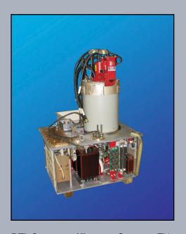
**DTI Compact Klystron System.** This system, rated at 21 kW average power, eliminates the need for a crowbar and provides thousands of hours of reliable operation.
