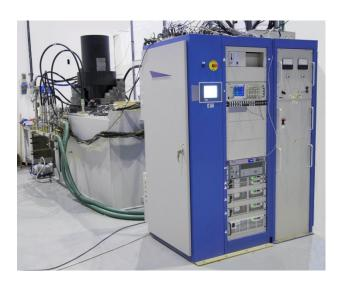
Fig. 1. Installed Daresbury modulator, consisting of a controls rack, electronics rack, high voltage power supply and modulator tank
