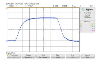
Fig. 4. Daresbury system pulse into a resistive load. Pulse is 350 kV (40 kV/V) for 3.5  $\mu$ s with less than .01% voltage flatness.
