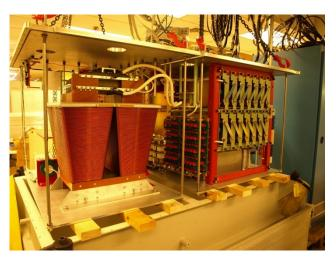
Fig. 2. The LBNL unit suspended above tank. On the left is the tapered pulse transformer; on the right, diodes and solid-state switch array. Far right: power supply cabinets.
