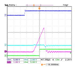
Fig. 5. Arc test for a DTI modulator. Channel 3 is the current at 100 A/div; Channel 4 is the detected fault; time scale is 1  $\mu$ s/div. The current is interrupted 800 ns after the fault is detected.
