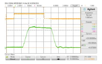
Fig. 3. Test pulse of LBNL system. Pulse is 275 kV, 250 A, with  $8\mu s$  command pulse.
