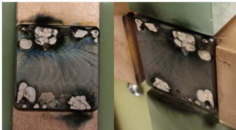
Figure 5. Left: Fast Mechanical Switch flexible copper strap side, with copper-tungsten insert. Right: Fixed side copper-tungsten contact area. Both photographs are after ~30 shots and show a little damage.
