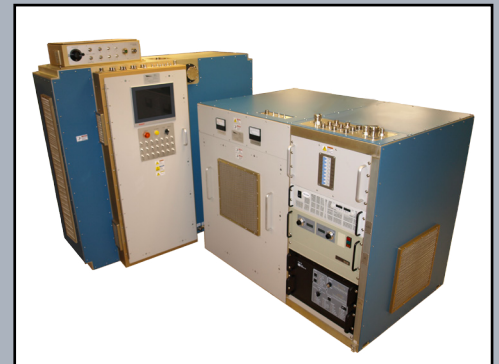
TWT Transmitter, comprised of the TWT cabinet (left) and capacitor bank cabinet (right). The TWT cabinet houses the TWT, high voltage switch, controls and auxiliary power supplies. The capacitor cabinet houses the high voltage capacitor bank, high voltage power supplies and power distribution unit.
