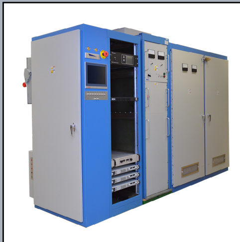
Klystron Test Stand showing controls and auxiliary supplies (left two cabinets), the high voltage power supply (center cabinet), and high voltage modulator (right two cabinets).
