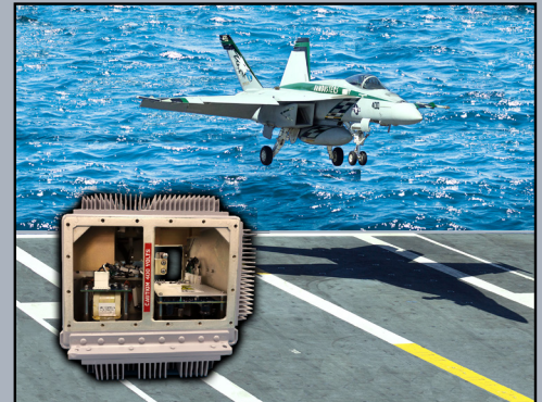
Magnetron Transmitter Upgrade for the US Navy's AN/SPN-41, used as a critical backup landing aid on aircraft carriers. Over 100 units delivered to date.
