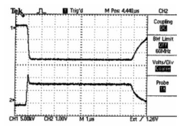
Figure 6: AN/SPG-60 Pulse, 13.5kV, 25 kHz, 8 µs
