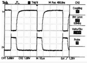
Figure 4: AN/SPG-60 train, 15kV, 25 kHz, 8 µs
