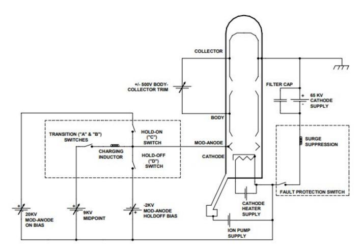
Figure 8: Schematic of NRL gyroklystron modulator.
