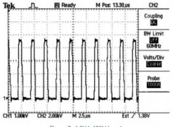
Figure 7: 4.5kV, 400kHz pulse
