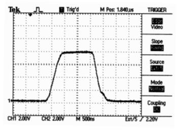
Figure 5: Transmitter pulse 8kV, 100kHz, 1.5µs
