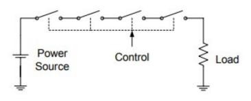
Figure 2: Solid state modulator components. The switches are in series.
