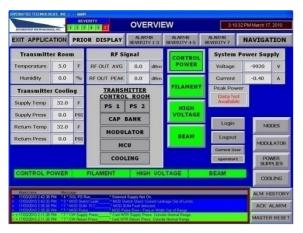
Figure 6. Screen shot of the transmitter overview touch screen control.
