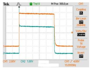
Figure 4. Scope shot of 100 kV pulse into resistive load, 520 µsec Ch1 Vk 99 kV (10 kV/div); Ch2 Ik 41A (10A/div).
