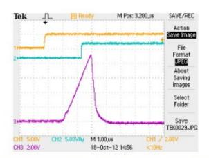
Figure 3. Simulated Arc. The fault occurs at 246 A. The switch opens in 690 ns; current peaks at 365 A.
